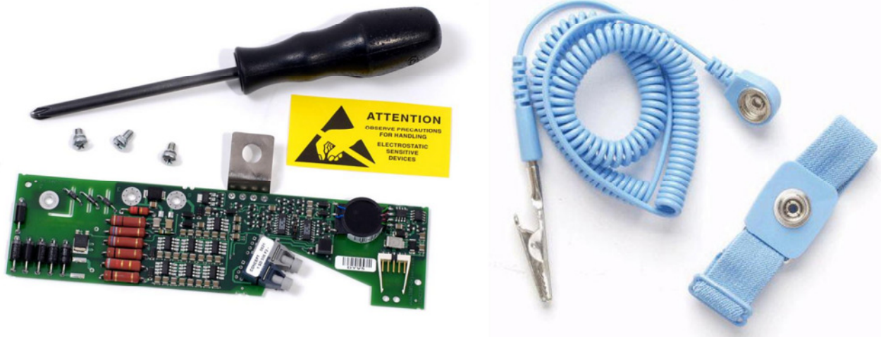
Fig. 2 ESD screwdriver and ESD wrist strap
